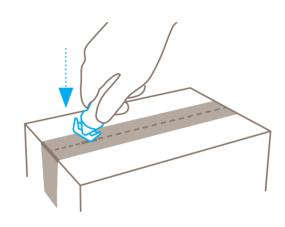
Pierce into cardboard adhesive tape using the flat edges on top of the blade head.
