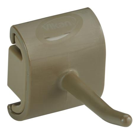
The single hook module is designed for hanging cleaning tools with a hanging hole. The hook is slid onto the supplied single-base/spacer from the left or right side. The single hook module can hold products weighing up to 3 kg. The hook is easy to disassemble for cleaning or replacement.
